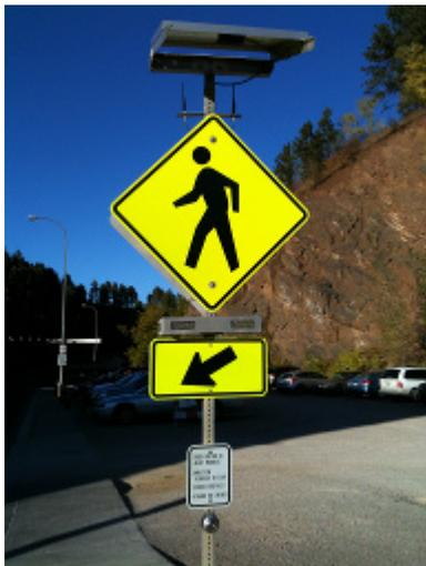
Rectangular Rapid Flashing Beacon (RRFB) with MUTCD Non Vehicular Warning Sign W11-2
