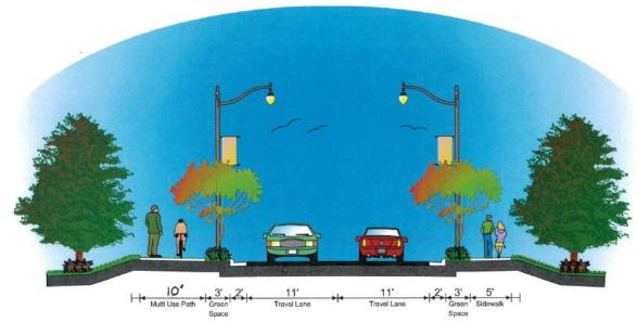
TWO-LANE ROAD WITH MULTI-USE PATH AND SIDEWALK 45-Foot Minimum Right-of-Way
